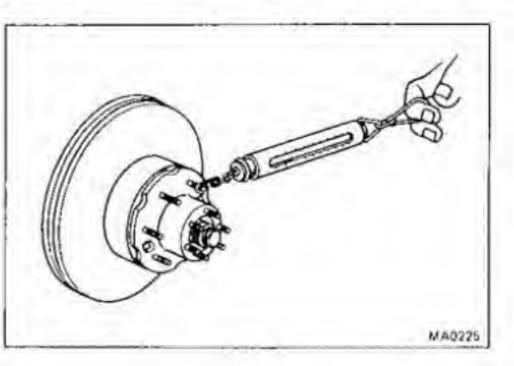
· Using a spring tension gauge, check for correct preload.
